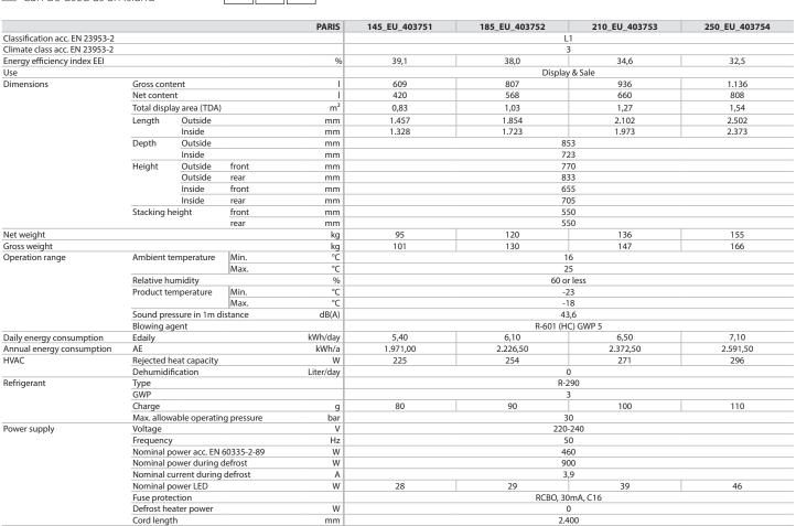
With process-related interior fitting | Energy test results are declared for climate class 3, test procedure according to EN 23953-2 (initial door openings, 12h LED switched on with door openings, one defrost per day) Chiller cabinets only on request
