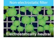
Because it catches particles relying only on mesh size, it is necessary to make mesh finer, making it easy to be clogged and cause high pressure loss.
