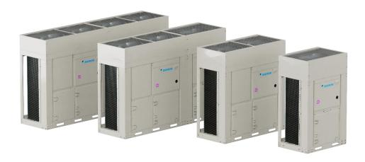
The EWYE-CZ offers heating in various applications and allows to produce domestic hot water. The range is available in 8 sizes from 16 kW to 70 kW, all equipped with Daikin Inverter Scroll Compressor technology. The operating range provides hot water temperatures from 20°C to 70°C, effectively functioning under diverse environmental conditions and operates in ambient temperatures ranging from -25°C to 40°C. Additionally, it can function with a significant temperature difference between the
