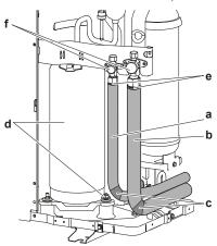
5 If the outdoor unit is installed above the indoor unit, cover the stop valves (f, see above) with sealing material to prevent condensed water on the stop valves from moving to the indoor unit.
