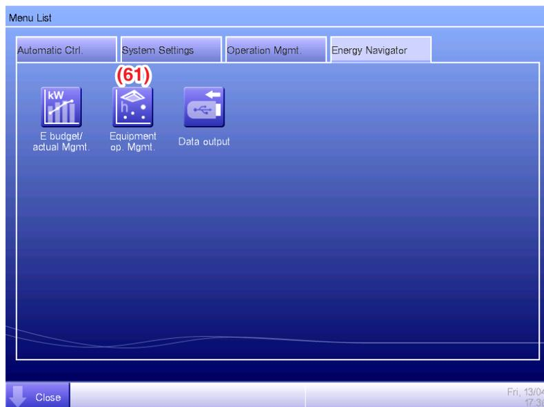
Touch the **Equipment op. Mgmt.** button (61) and display the Equipment operation management screen. The Equipment operation management screen consists of two tabs: Failure to turn off and Setpoint gap.
