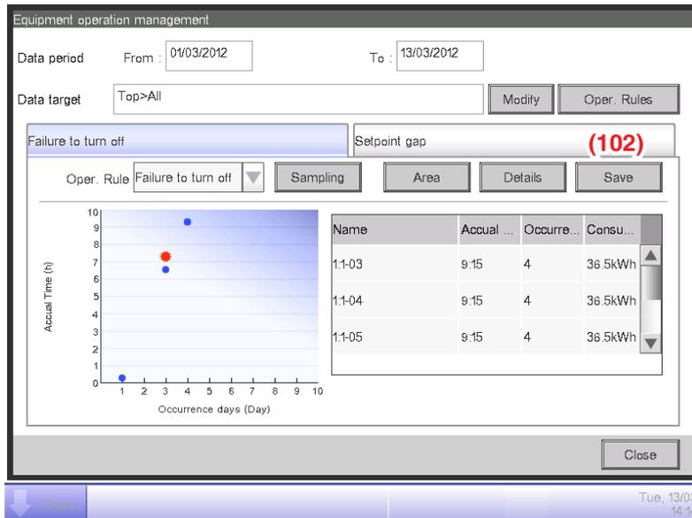
Connecting a USB memory to the iTM unit and touching the **Save** button (102) saves the data sampled using the conditions displayed on the current screen to a CSV file.
