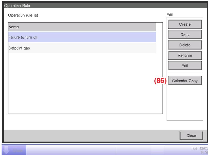
Select the operation rule where the calendar to copy is registered and touch the **Calendar Copy** button (86) to display the Calendar Copy screen.
