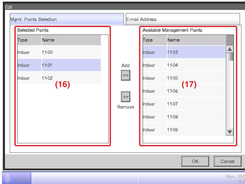
(16) is the list of management points registered as target of error monitoring while (17) is the list of management points that can be registered. To register, select a management point that will be target of monitoring from (17) and touch the Add button. You can register up to 512 management points. Selecting a management point from (16) and touching the Remove button cancels its registration.
