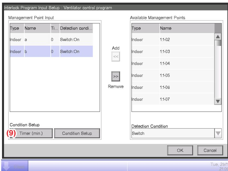
Select the indoor unit “a” and touch the **Timer (min.)** button (9) and enter “10” for required duration in the Numerical Input dialog that appears.
