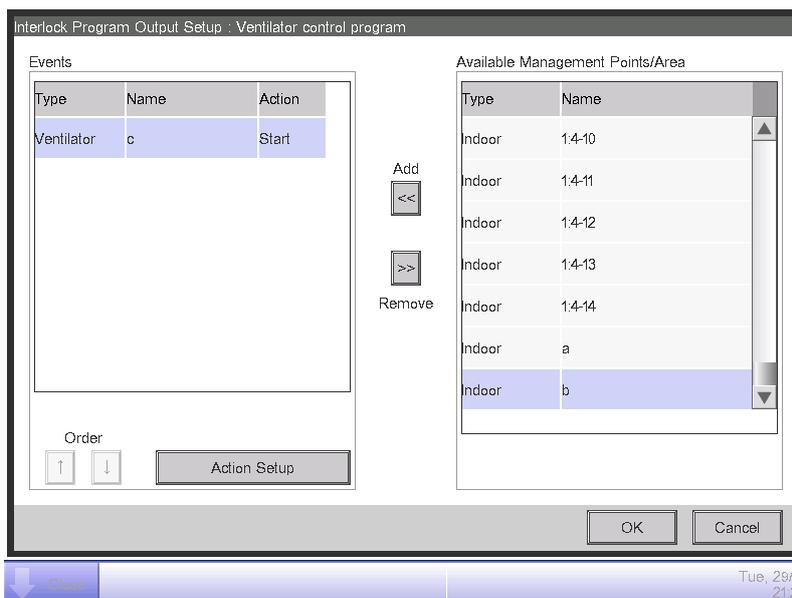
Touch the OK button and return to the Interlock Program Setup screen.
