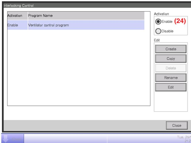
Select “**Ventilator control program**” and select the **Enable** radio button (24).
