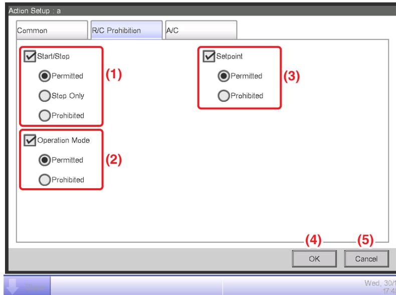
Select the check box of the items to set up and select the setting using the radio buttons.
