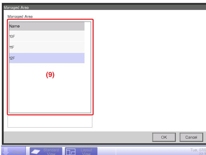
(9) is the list of areas that can be registered. Select one area and touch the OK button to save the settings and return to the User Setup screen.
