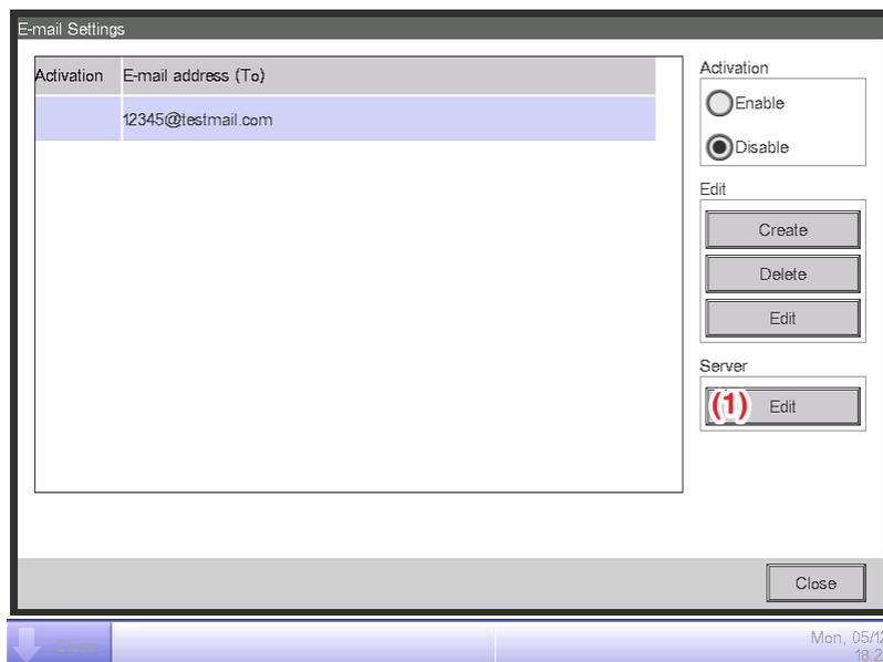
Touch the **Edit** button (1) and display the Server dialog. The dialog consists of two tabs: Transmission and E-mail Server. Switch and set up each of the tabs. When finished, touch the OK button to save and return to the E-mail Settings screen.
