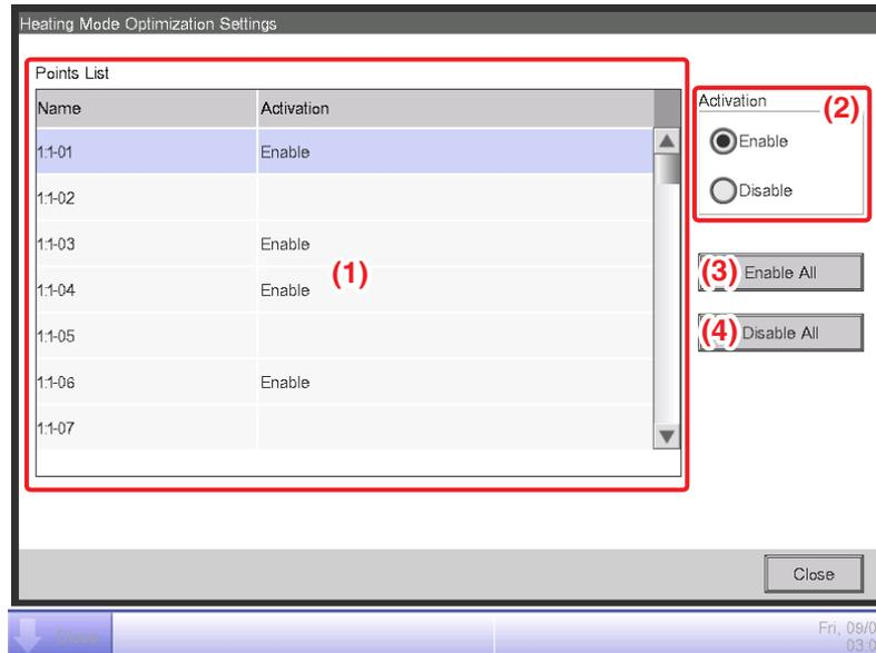
2. Select an indoor unit from list (1) displaying the names of indoor units and whether this function is enabled or disabled, and then select Enable or Disable in (2).
