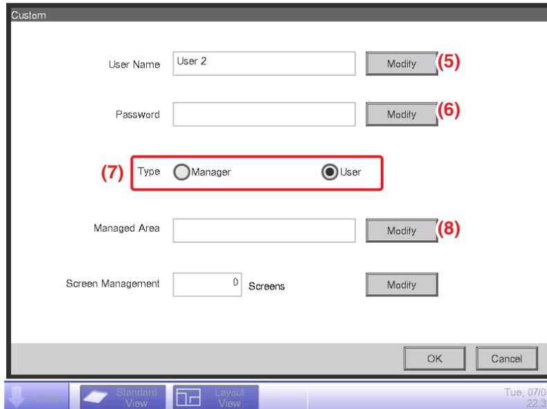
To enter the user name, touch the **Modify** button (5) and display the Text Input dialog. Specify a name using 1 to 15 characters, irrespective of single or double byte.
