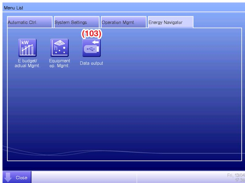
Touch the **Data output** button (103) and display the Data output screen. The Data output screen consists of two tabs: Energy Data and Mgmt. Point Data
