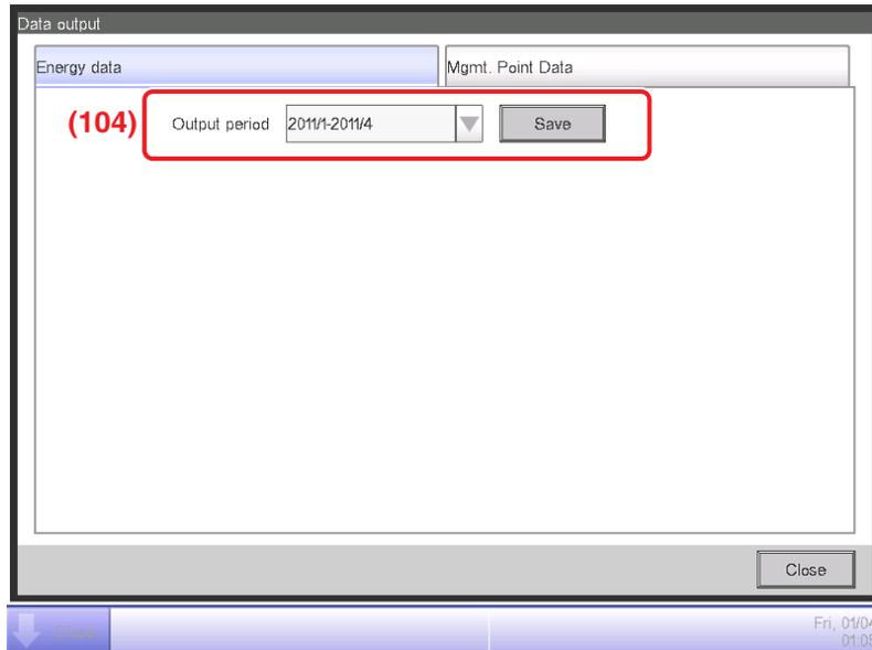
In the **Output period** combo box **(104)**, select the data to output from This year and Last year. Connect a USB memory to the iTM unit and touch the Save button. Touching the OK button on the confirmation dialog that appears starts the output.
