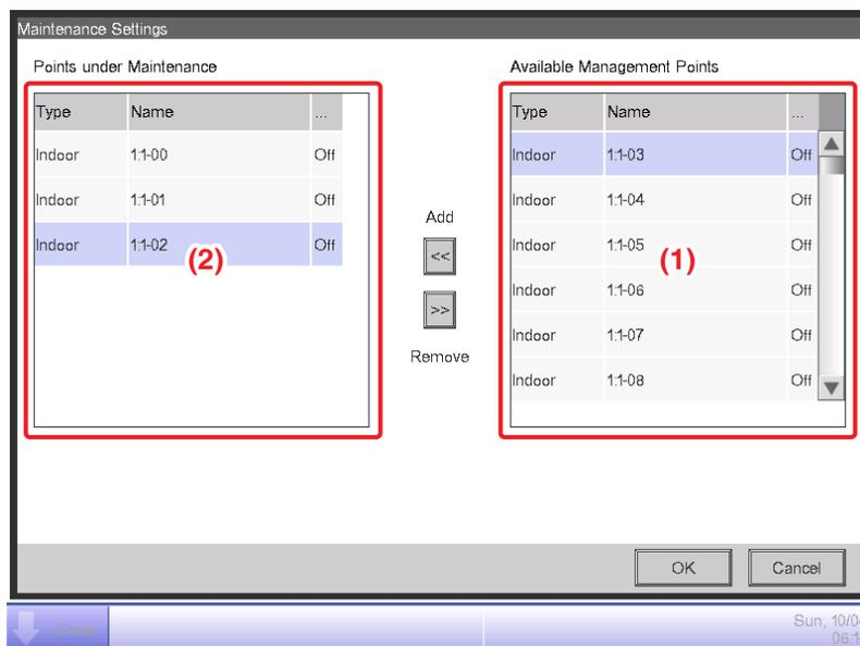
2. To set to maintenance, select a management point from (1) and touch the Add button to move it to (2). The management point is set to maintenance. Touch the OK button to save and close the screen.
