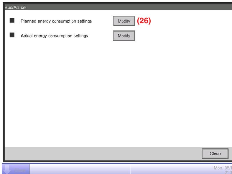
Touch the **Modify** button (26) and display the Planned Energy Consumption Setup screen.
