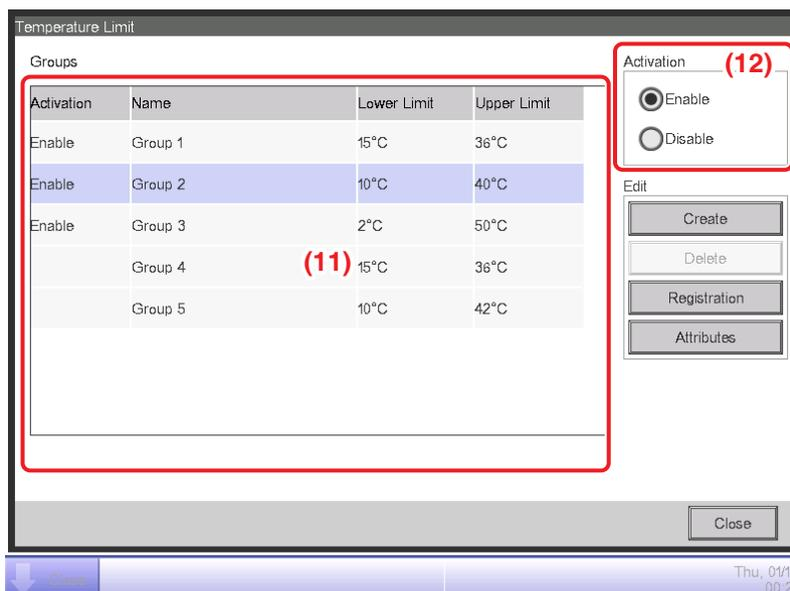
5. To enable the Temperature Limit function for the group selected in (11), select the Enable in the Activation radio button area (12) button. To disable, select the Disable button.
