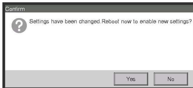
5. A restart confirmation message will be displayed. Touch the Yes button to reflect the setting and restart the iTM.
