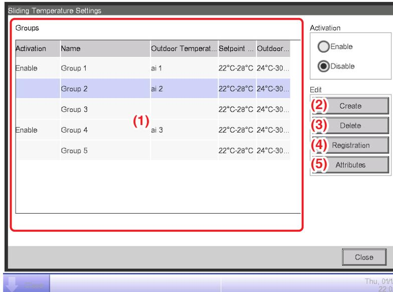
2. (1) is the list of Sliding Temperature groups. Perform the intended operation by touching the relevant button on the right.
