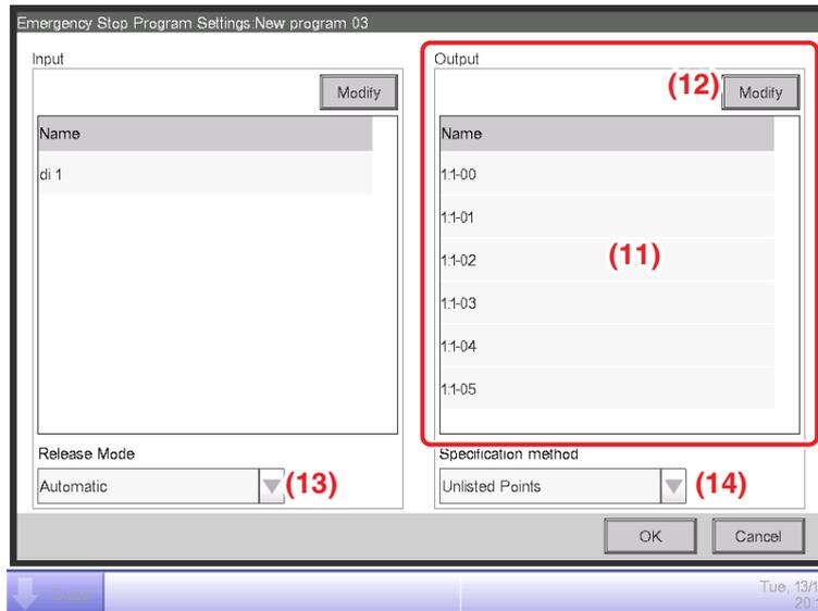
6. (11) is the list of management points target of the Emergency Stop. Touch the **Modify** button (12) and register management points, as in step 5.
