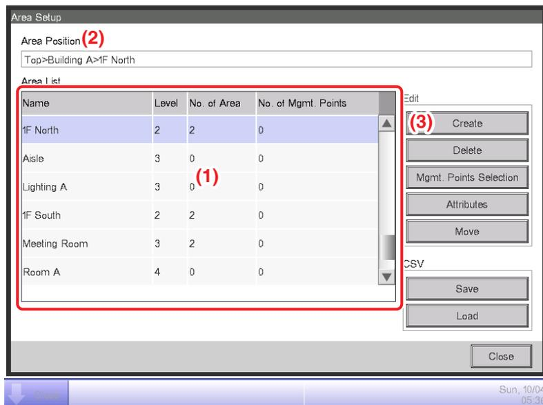
2. (1) on the Area Setup screen is the list of areas displayed as a tree structure organized in descending order. Select the higher level area (for example, 1F North) into which to create the new one. (2) indicates the position of the currently displayed area (for example, Top>Building A>1F North).
