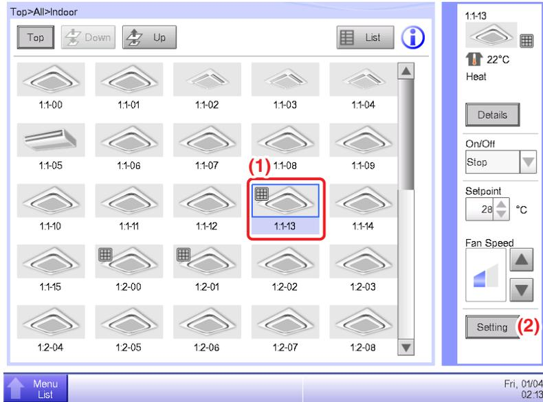
1. Select **(1)** with the filter sign ON on the Standard View screen and touch the **Setting** button **(2)** to display the Detailed Setup screen.
