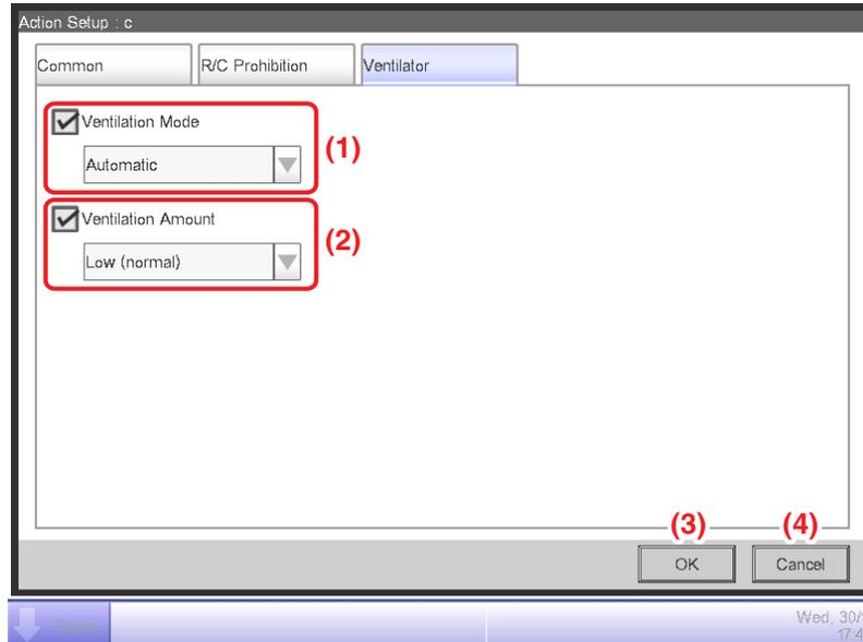
Select the check box of the items to set up and select the setting from the combo box.
