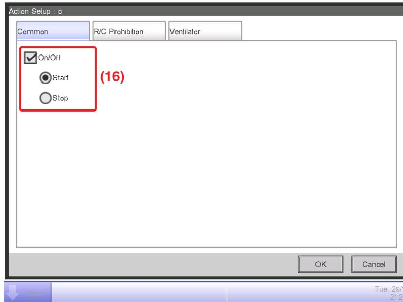
Select the **On/Off** check box **(16)** on the Common tab and then, select the **Start** radio button. Touch the OK button and return to the Interlock Program Output Setup screen.
