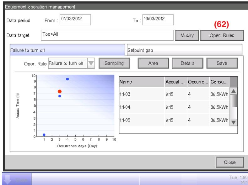
Touch the **Oper. Rules** button (62) and display the Operation Rule screen. The Oper. Rules button is available on both tabs.
