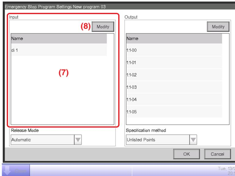
4. **(7)** is the list of management points input as emergency stop signal. Touch the **Modify** button **(8)** and display the Management Points Selection screen.
