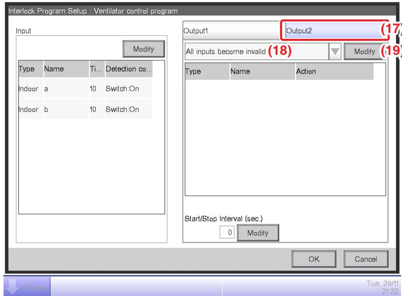
The step above finishes the setup of **Output1** for the program, “which turns on Ventilator “c” when either indoor unit “a” or “b” is On for 10 minutes”.
