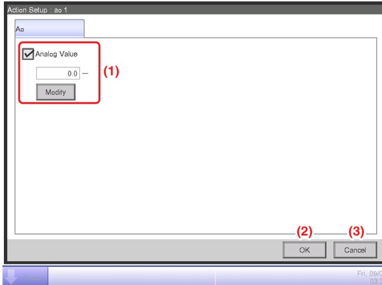
Select the check box of the items to set up and enter the setting using the Modify button.
