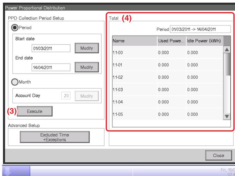
Touching the **Execute** button **(3)** displays a confirmation dialog. Connect the USB memory to the iTM unit and touch the Yes button to start data collection and CSV file output.
