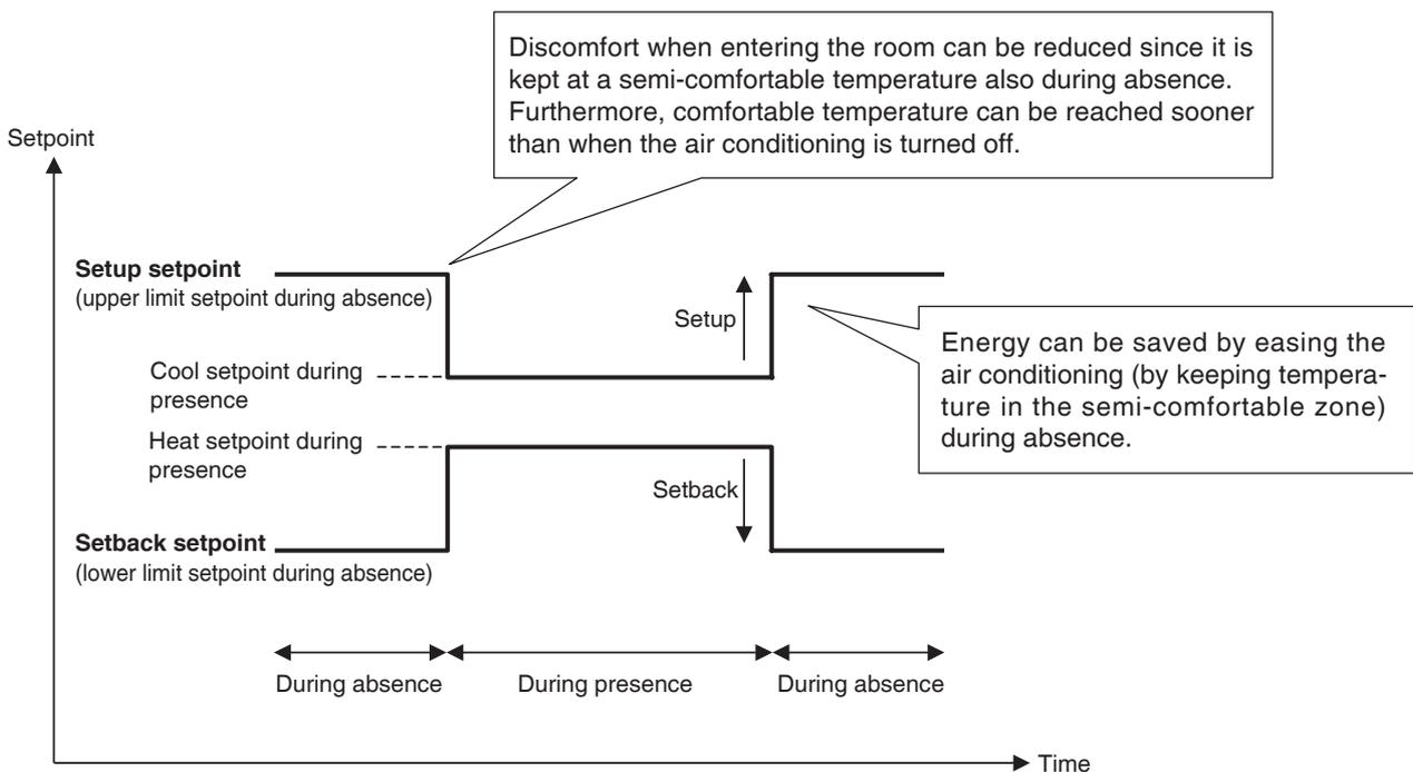
Indoor units and areas where this function is enabled are controlled as follows.
