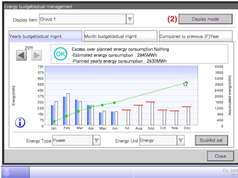
Touch the **Display mode** button (2) and display the Display mode screen. The Display mode button is available on all tabs.
