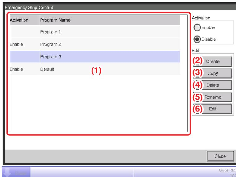
2. (1) is the list of emergency stop programs. Perform the intended operation by touching the relevant button on the right.
