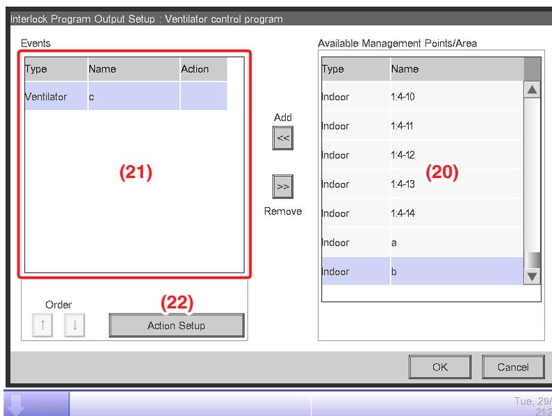
Select Ventilator “c” from (20) and touch the Add button to register it as target of the output event in (21).
