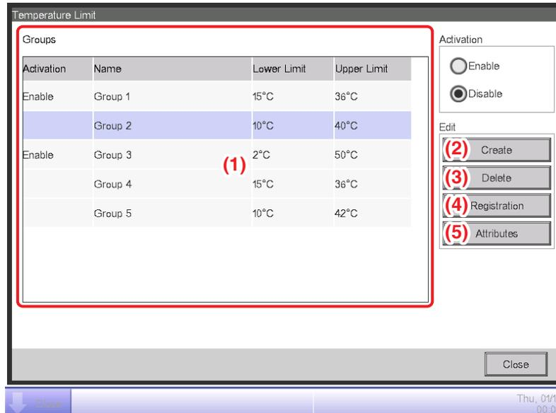
2. (1) is the list of Temperature Limit groups. Perform the intended operation by touching the relevant button on the right.
