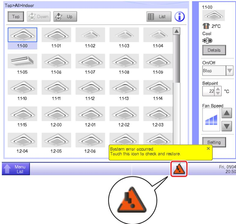
1. When an error is detected, it is notified by a flashing
