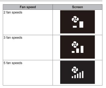
Some indoor units additionally support Automatic fan speed. In this case, the indoor unit adjusts its fan speed automatically, according to the setpoint and indoor temperature.
