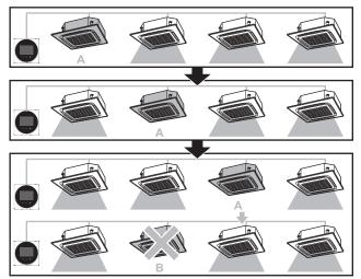
A Inactive backup unitB Unit in error
